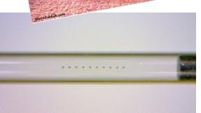
We are also able to control depth of the cut or hole by the number of laser pulses delivered to the surface. With UV lasers, this pulse control allows us to create very precise blind holes or wells in glass surfaces. In addition, lasers are also excellent tools for precision marking of glass for applications such as putting fiduciary marks on parts, or batch control codes.
